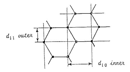
Figure 3.1: Structure of Graphite
