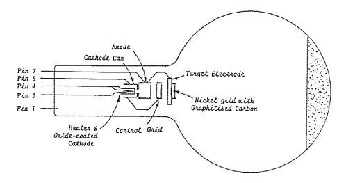
Figure 3.2: Schematic of the Electron Diffraction Tube
